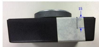
Figure 6 Marking the mounting location for the switch. Please see text for details.
