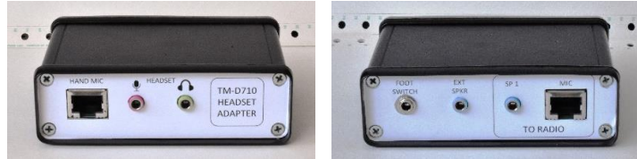
Front and rear panels of junction box
