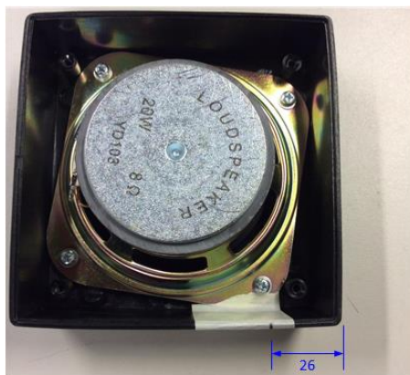
Figure 6 Marking the mounting location for the switch. Please see text for details.
